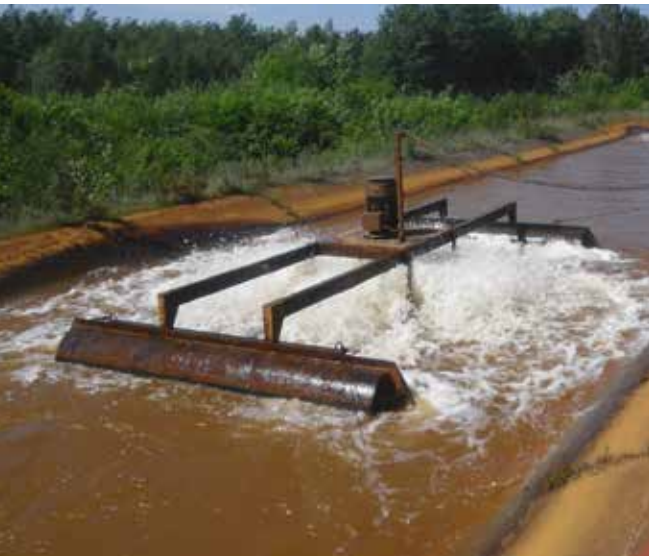
AeroStar Aerators on floats for stripping of carbon dioxide (Germany)
