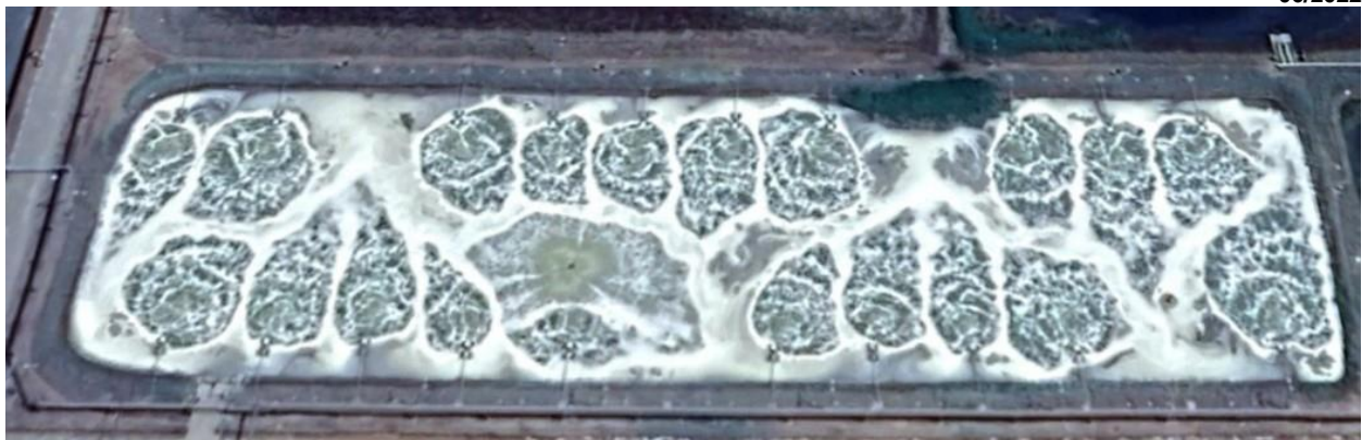
20 x FUCHS OS 30 (22 kW) and 2 x 55 kW Surface Aerators
